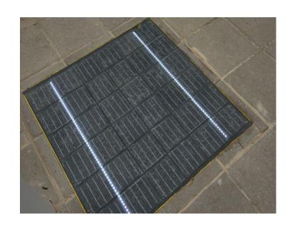
Environmental Technology of the Tallinn University of Technology School of Engineering: made a prototype of a smart road pavement what produces electricity from sunlight.
